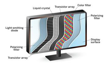
Liquid-crystal displays (LCDs) consist of multiple layers. Light produced by a light-emitting diode passes through polarizing filters, color filters, and a liquid-crystal layer to produce an image. Credit: Adapted from Shutterstock.
